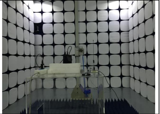
Radiated Spurious Emissions Test Setup Above
