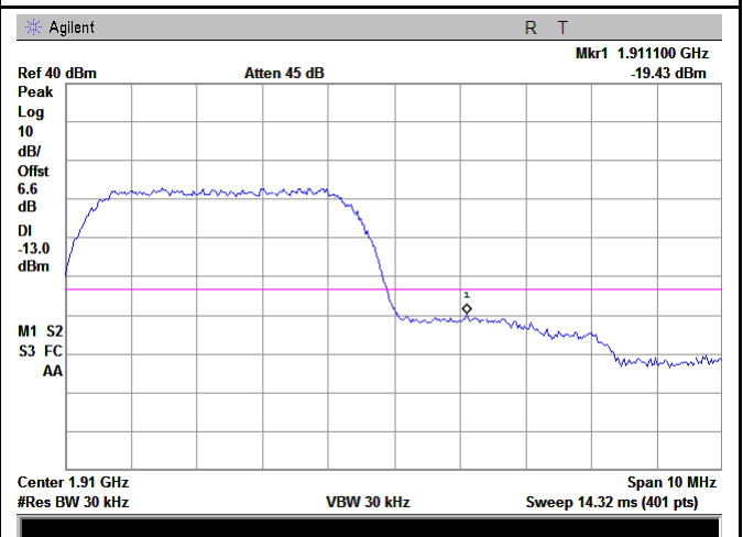
UMTS-FDD Band II - High Channel
