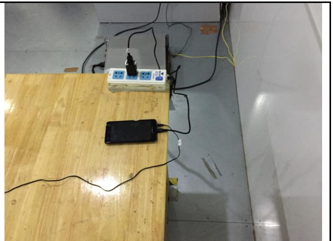
Conducted Emissions Test Setup Side View
