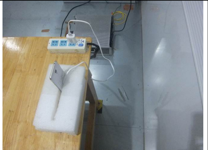
Conducted Emissions Test Setup Side View
