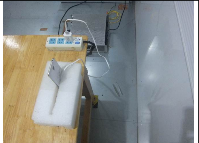
Conducted Emissions Test Setup Side View
