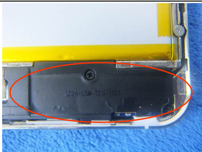
GSM/PCS/UMTS-FDD/LTE Antenna View
