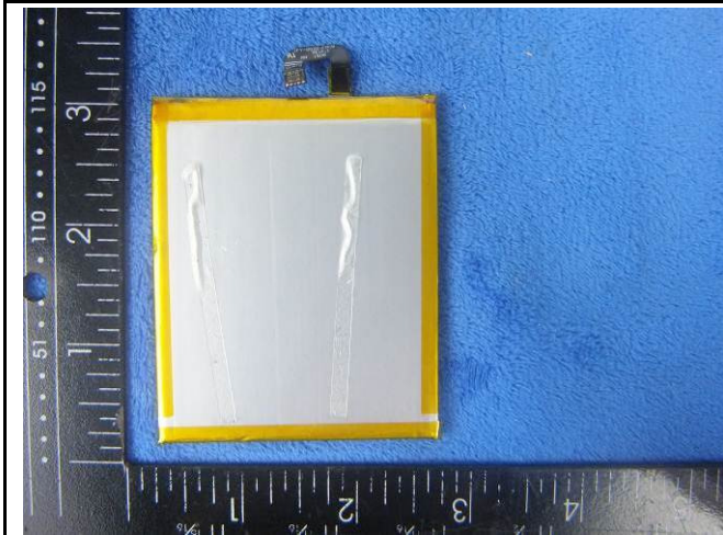
Battery - Rear View
