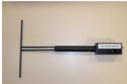
Figure 1 – Satimo COMOSAR Validation Dipole
