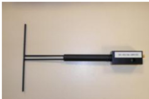
Figure 1 – Satimo COMOSAR Validation Dipole
