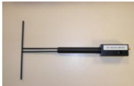
Figure 1 – Satimo COMOSAR Validation Dipole
