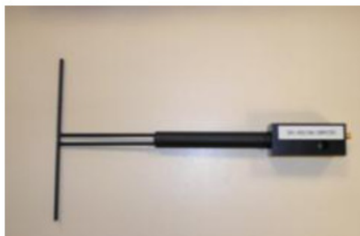
Figure 1 – Satimo COMOSAR Validation Dipole
