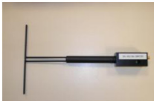
Figure 1 – Satimo COMOSAR Validation Dipole
