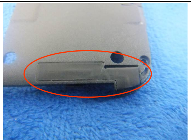
GSM/PCS/UMTS-FDD/LTE Antenna View
