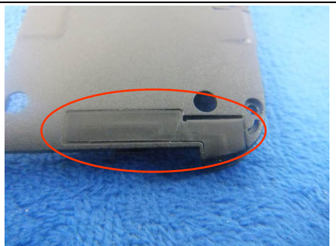
GSM/PCS/UMTS-FDD/LTE Antenna View
