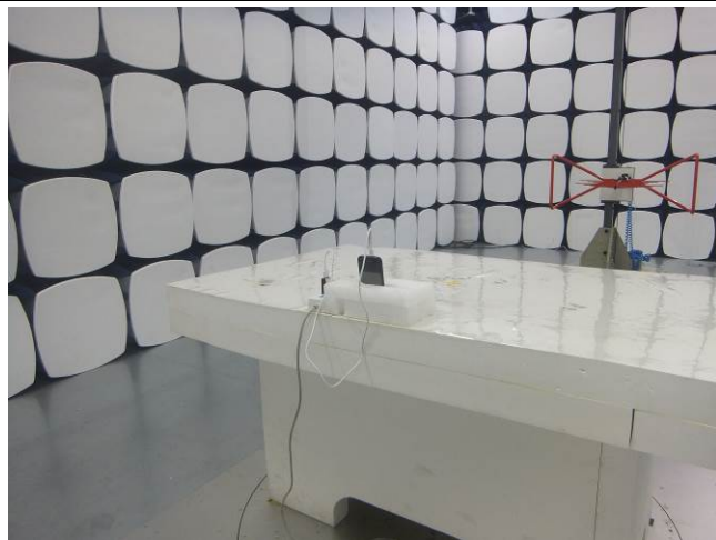
Conducted Emissions Test Setup Front View
