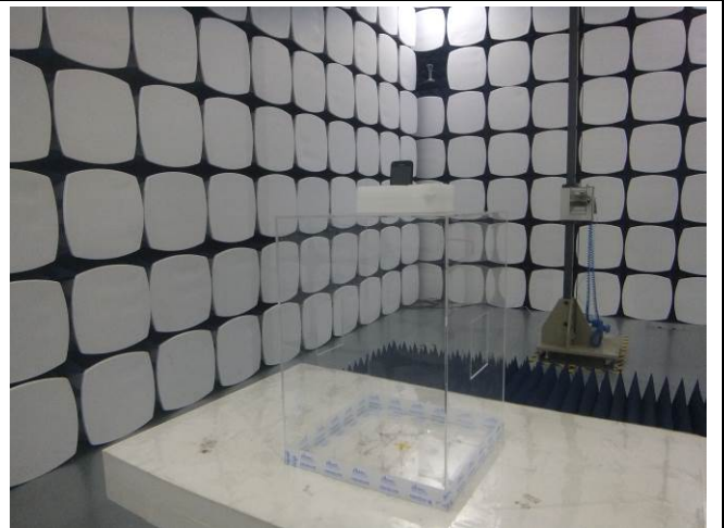
Radiated Spurious Emissions Test Setup Above 1GHz
