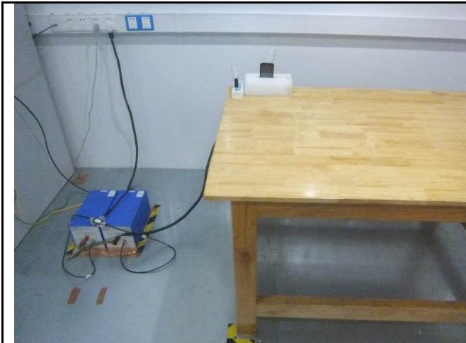
Conducted Emissions Test Setup Front View
