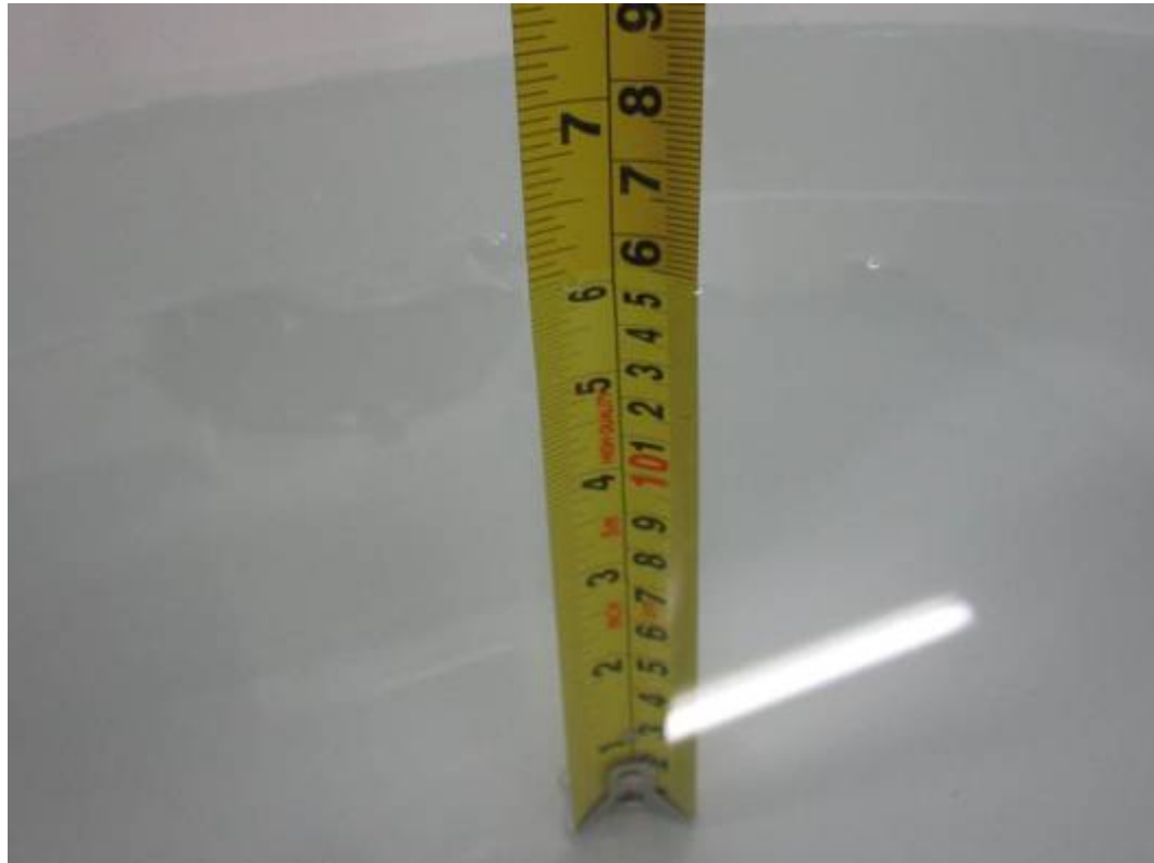
Liquid depth \geq 15\text{cm}
