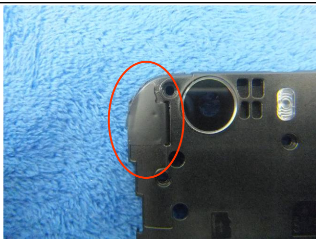
LTE - Antenna View
