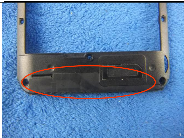
GSM/PCS/UMTS-FDD/LTE Antenna View
