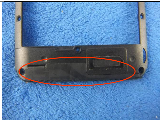
GSM/PCS/UMTS-FDD/LTE Antenna View
