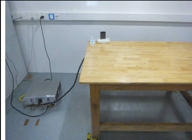
Conducted Emissions Test Setup Front View
