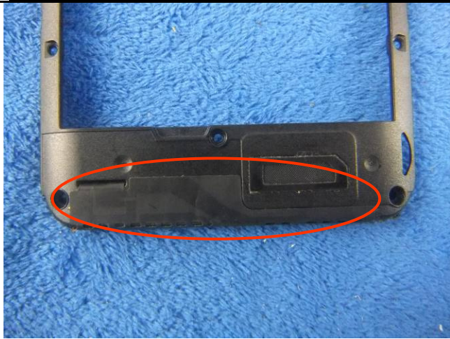
GSM/PCS/UMTS-FDD/LTE Antenna View
