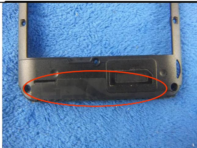
GSM/PCS/UMTS-FDD/LTE Antenna View
