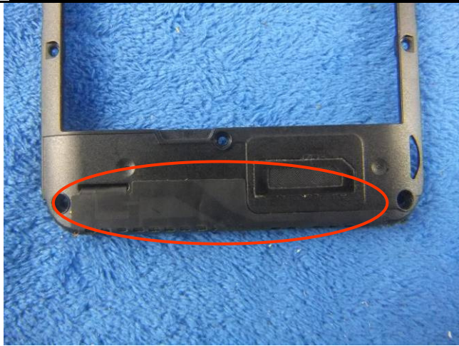
GSM/PCS/UMTS-FDD/LTE Antenna View
