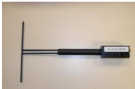
Figure 1 – Satimo COMOSAR Validation Dipole
