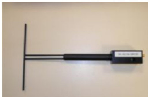
Figure 1 – Satimo COMOSAR Validation Dipole
