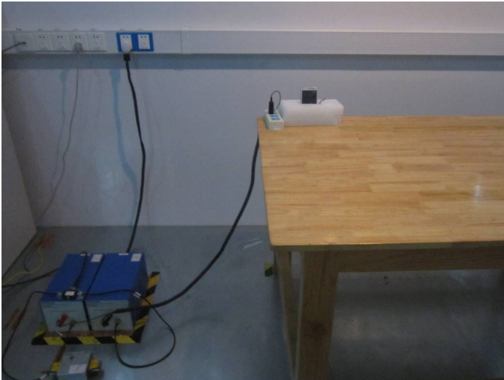
Conducted Emissions Test Setup Front View
