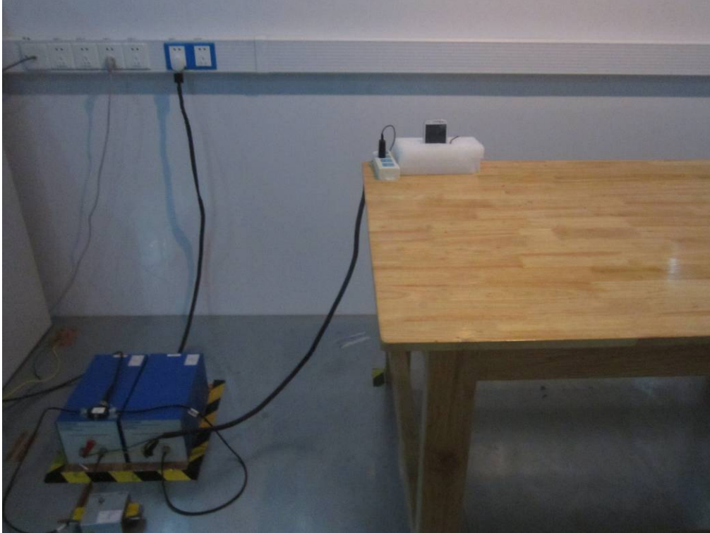
Conducted Emissions Test Setup Front View
