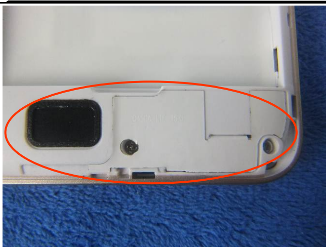
GSM/PCS/UMTS-FDD/LTE Antenna View
