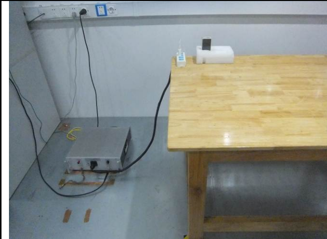
Conducted Emissions Test Setup Front View
