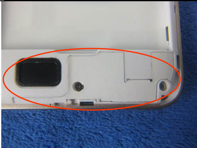
GSM/PCS/UMTS-FDD/LTE Antenna View
