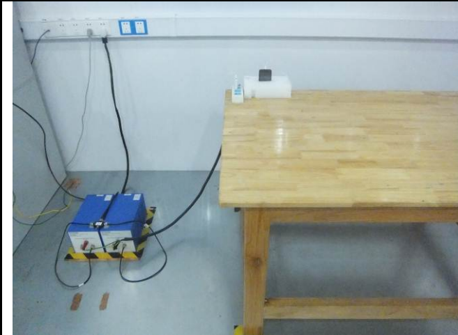
Conducted Emissions Test Setup Front View
