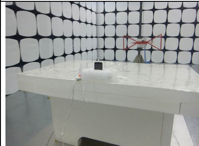
Conducted Emissions Test Setup Front View
