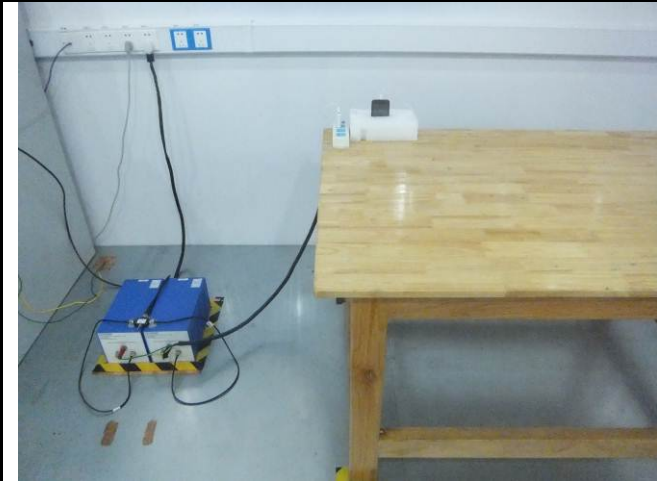
Conducted Emissions Test Setup Front View
