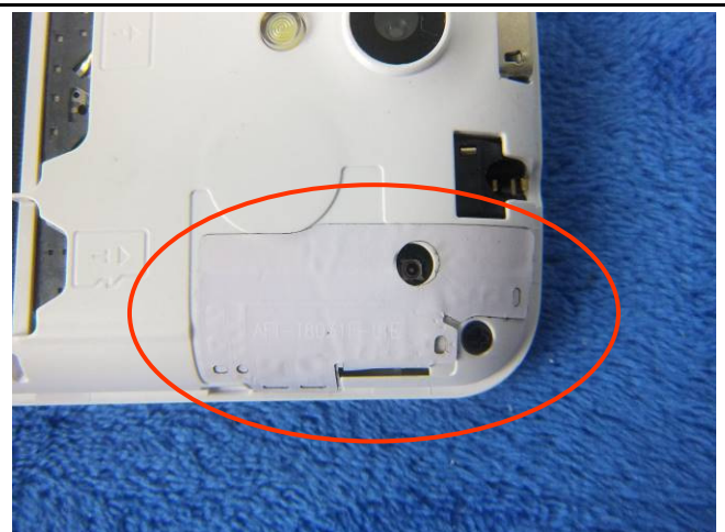
LTE - Antenna View
