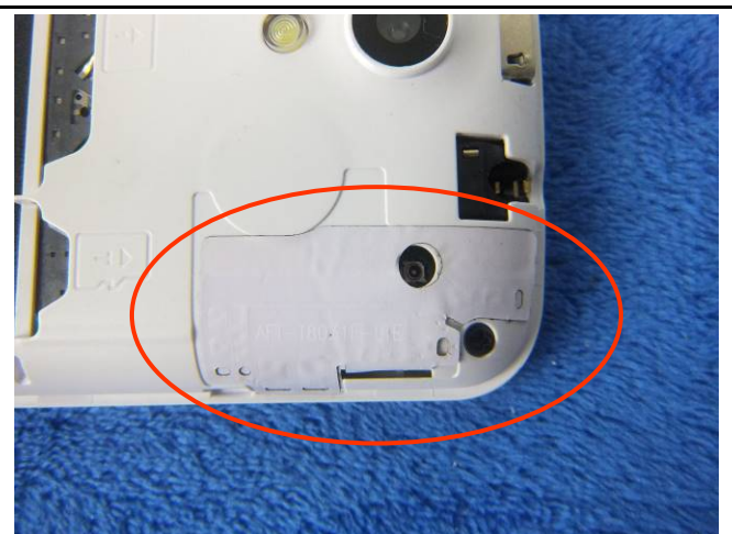
LTE - Antenna View
