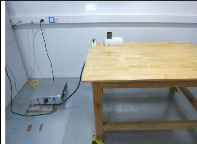
Conducted Emissions Test Setup Front View
