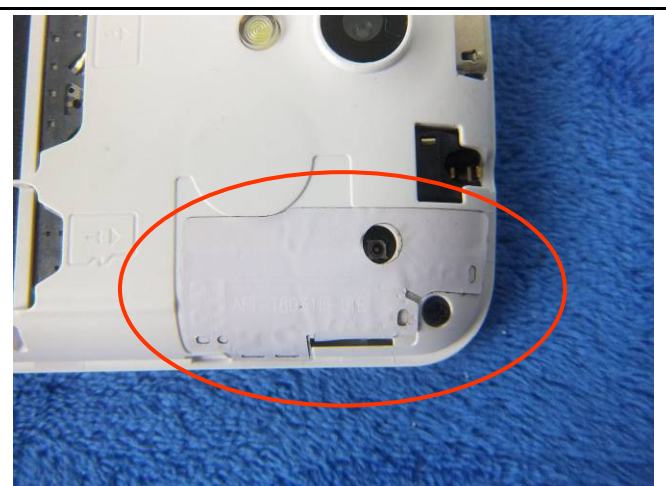
LTE - Antenna View
