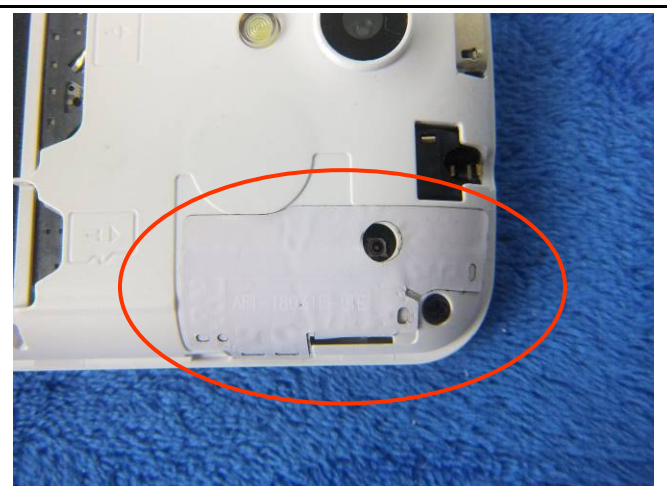
LTE - Antenna View
