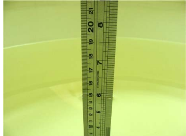
Fig 6.2 Photo of Liquid Height for Body SAR
