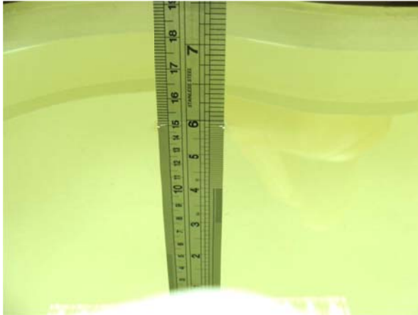
Fig 6.1 Photo of Liquid Height for Head SAR
