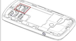
■ Finally, install the battery and cover the back cover of the mobile phone. Please keep your memory card safe.
