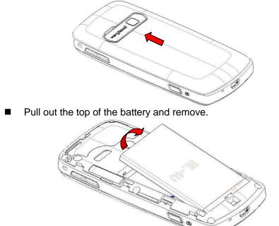
■ When installing the battery, insert the metal contact at the bottom of the battery into the corresponding slot of the mobile phone, and then press the battery down to install it in place. The battery must be
