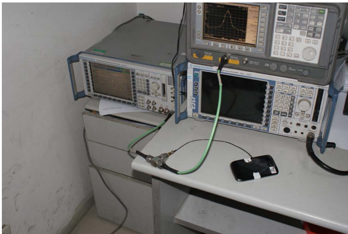
CONDUCTED TEST SETUP
