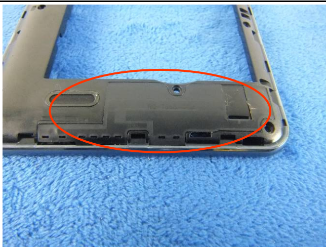
GSM/PCS/UMTS-FDD Antenna View
