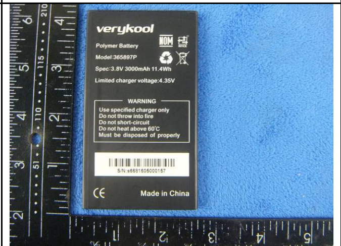
Battery - Rear View
