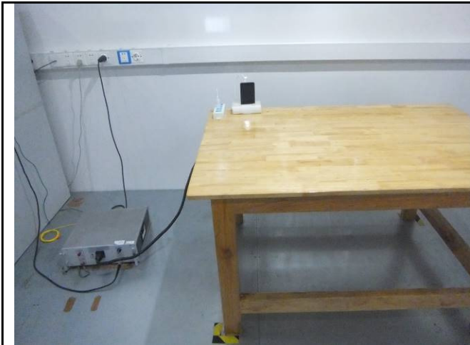
Conducted Emissions Test Setup Front View
