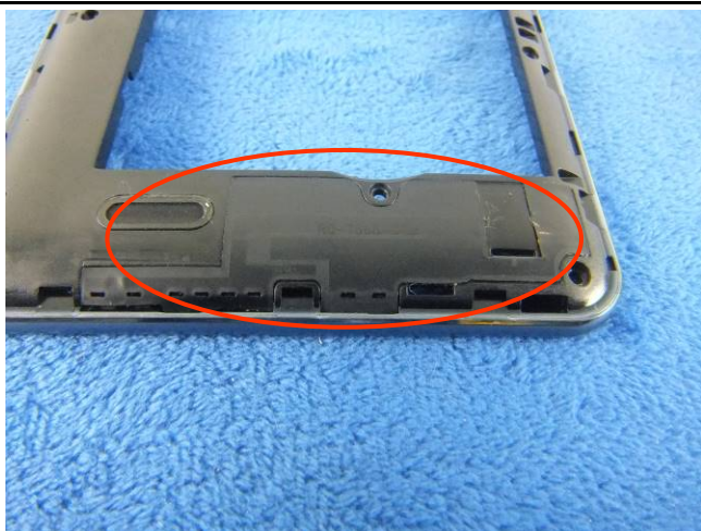
GSM/PCS/UMTS-FDD Antenna View
