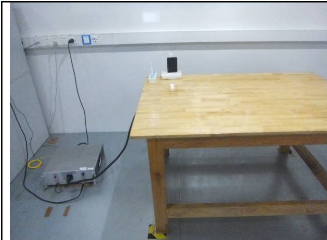
Conducted Emissions Test Setup Front View
