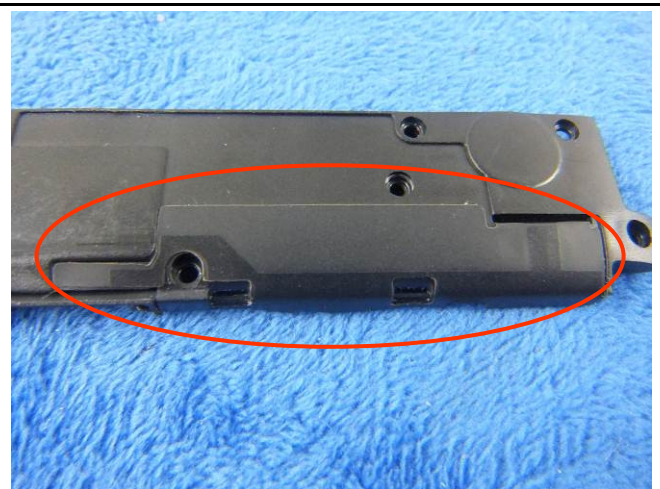
GSM/PCS/UMTS-FDD Antenna View
