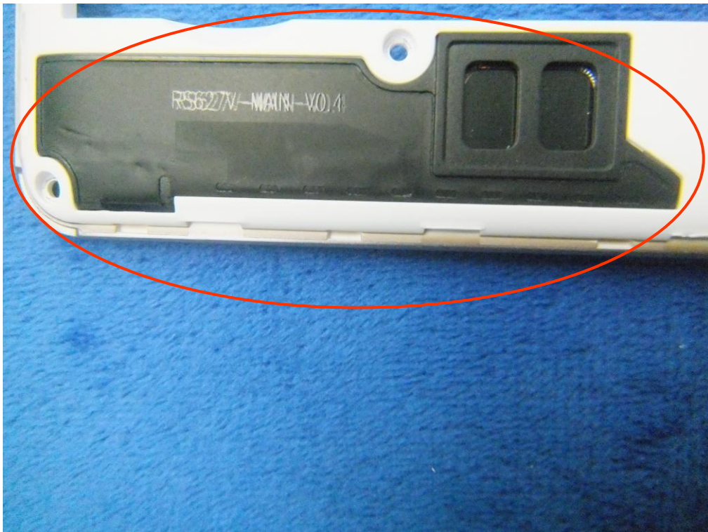
GSM/PCS/UMTS - Antenna View
