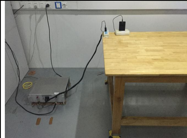
Conducted Emissions Test Setup Front View
