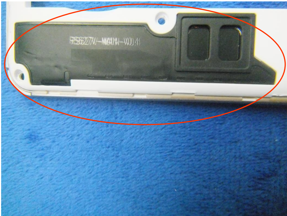
GSM/PCS/UMTS - Antenna View
