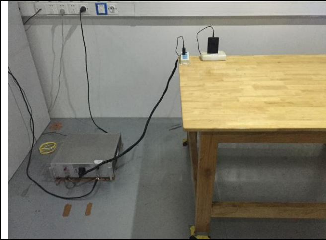
Conducted Emissions Test Setup Front View
