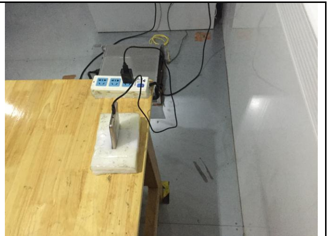
Conducted Emissions Test Setup Side View
