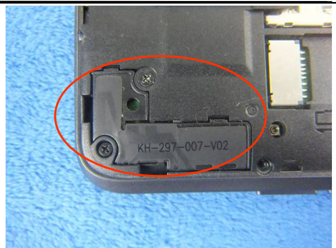
WIFI/BT/BLE/GPS - Antenna View
