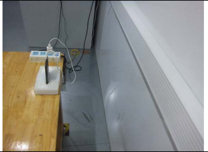
Conducted Emissions Test Setup Side View
