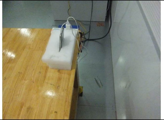
Conducted Emissions Test Setup Side View
