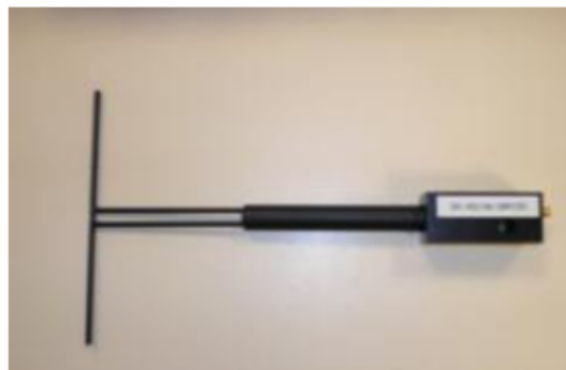
Figure 1 – Satimo COMOSAR Validation Dipole
