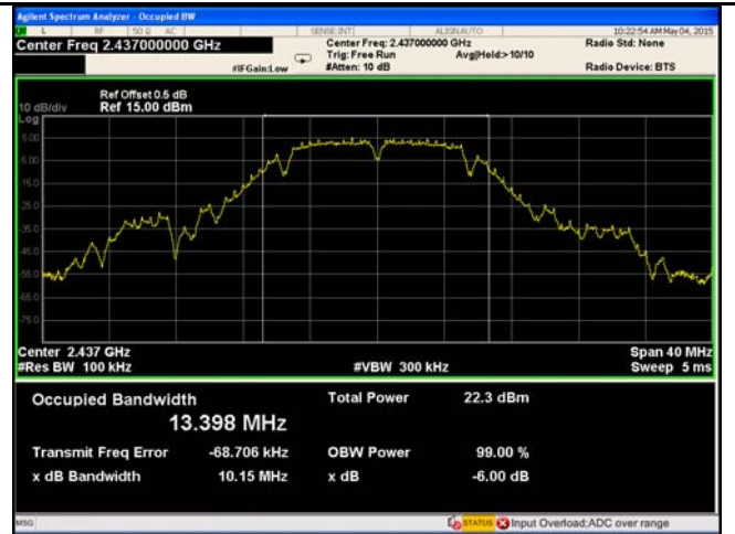
802.11b 6dB Bandwidth - Mid CH 2437
