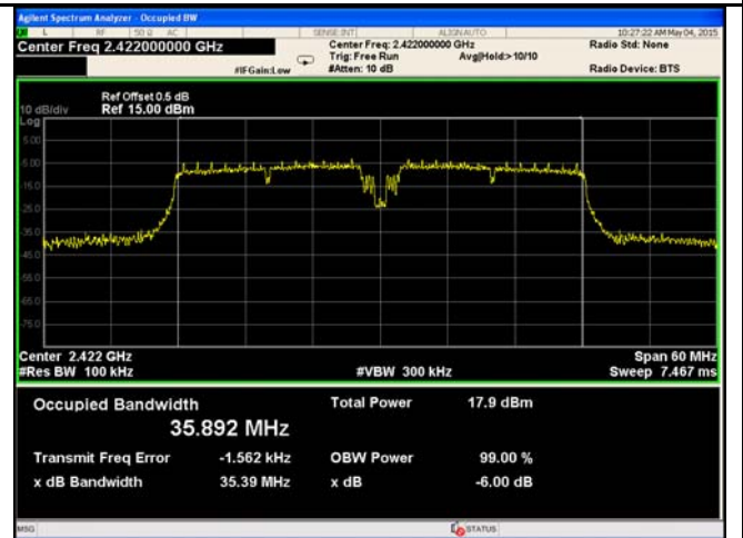
802.11n40 6dB Bandwidth - Low CH 2412
