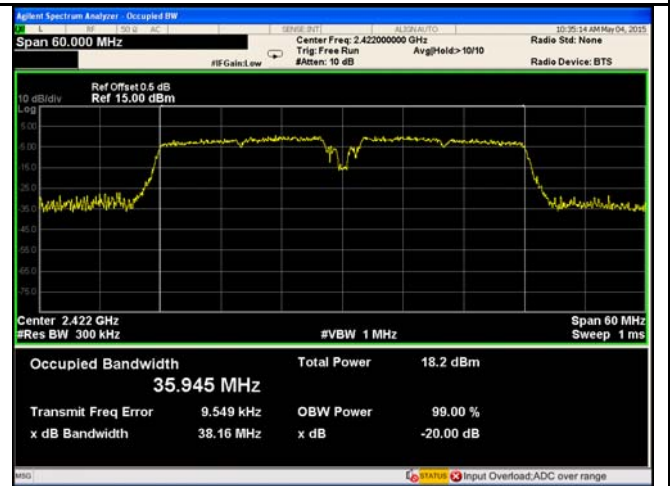
802.11n40 20dB Bandwidth - Low CH 2412
