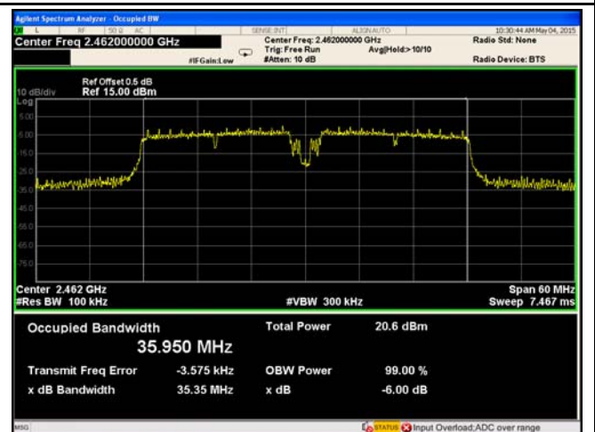
802.11n40 6dB Bandwidth - High CH 2462
