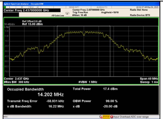
802.11b 20dB Bandwidth - Mid CH 2437
