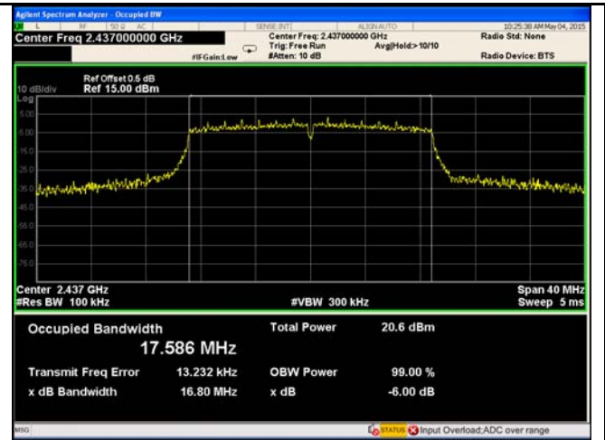
802.11n20 6dB Bandwidth - Mid CH 2437
