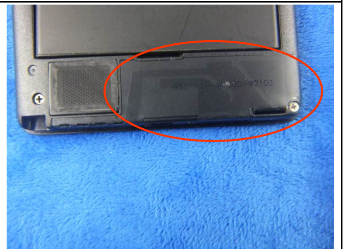
GSM/PCS/UMTS-FDD Antenna View
