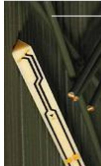
Construction Symmetrical design with triangular Core. Built-in shielding against static charges Calibration in air from 100 MHz to 2.5 GHz. In brain and muscle simulating tissue at frequencies from 800 to 6000 MHz (accuracy of 8%) .
