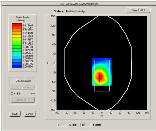
Test mode: WCDMA Band V, Middle channel (Left Head Cheek)
