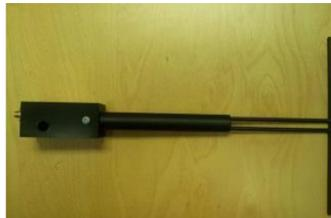
Figure 1 – MVG COMOSAR Validation Dipole
