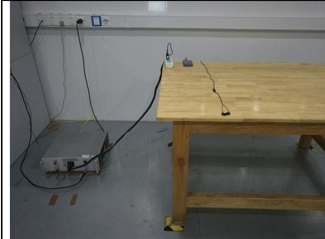
Conducted Emissions Test Setup Front View
