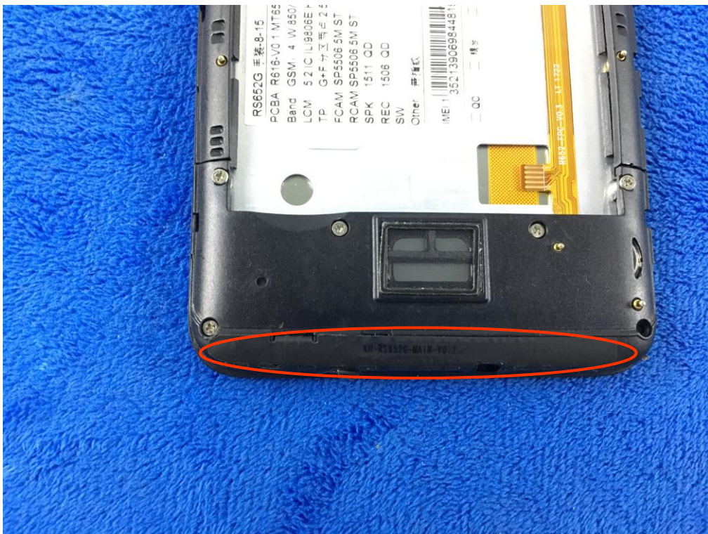
GSM/PCS/UMTS-FDD Antenna View
