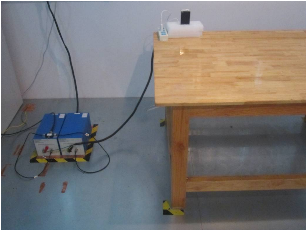
Conducted Emissions Test Setup Front View
